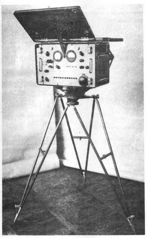
The instrument is mounted on it's own tripod with a turnable and tiltable head for slope measurements when required.
