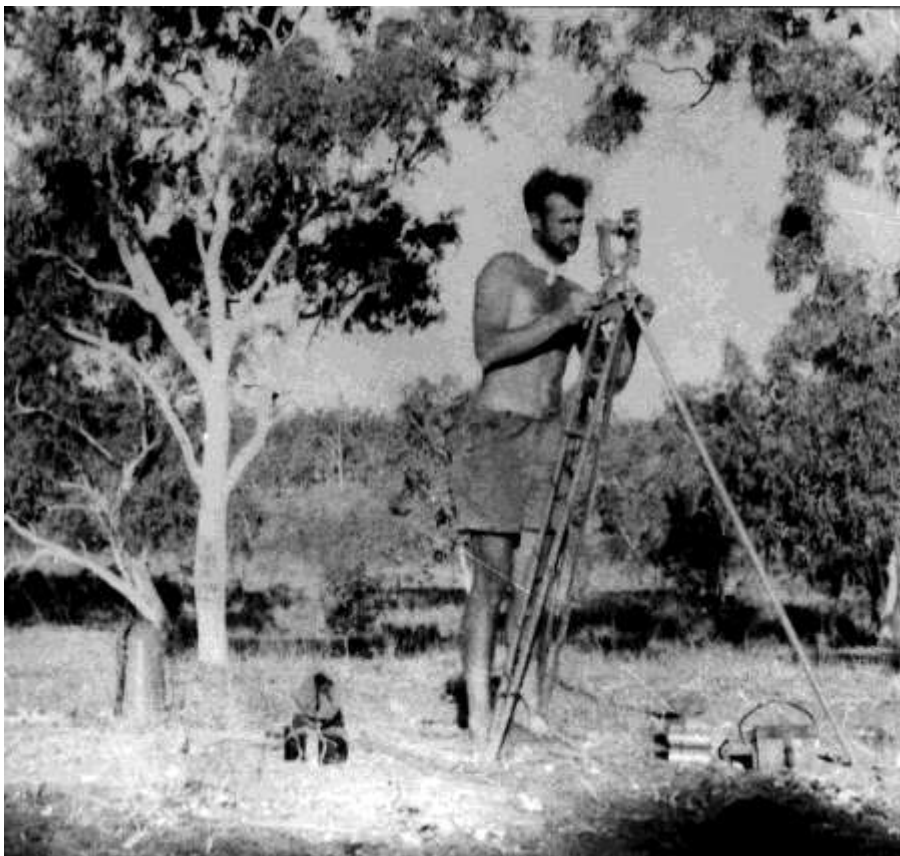
Figure 2. Setting up for the Astrofix observation at Bluey W.H., Station NMH100, between Robinson River and Calvert Hills Homesteads, 1949.
