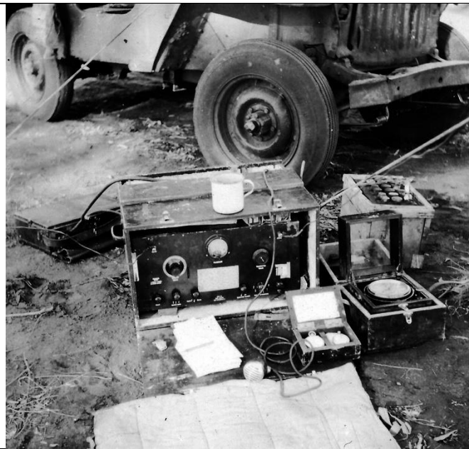
AWA 3BZ transceiver with watches and chronometer set up for time check
