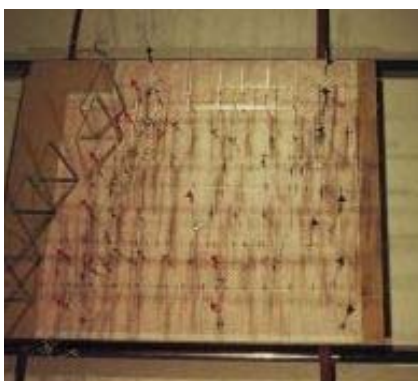
The Jerie ITC Analogue Computer c1963 for Height (left) and Positional (right) Adjustment of Blocks of Aerial photography.
