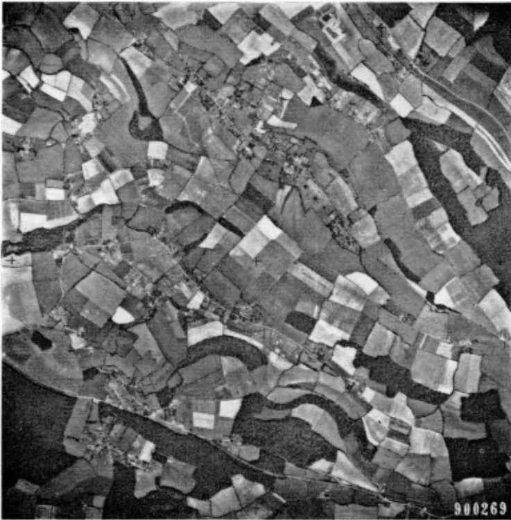
FIG. 1.4. A CONTACT PRINT (shown reduced from 230 mm × 230 mm) ( Fairey Surveys Ltd. )
