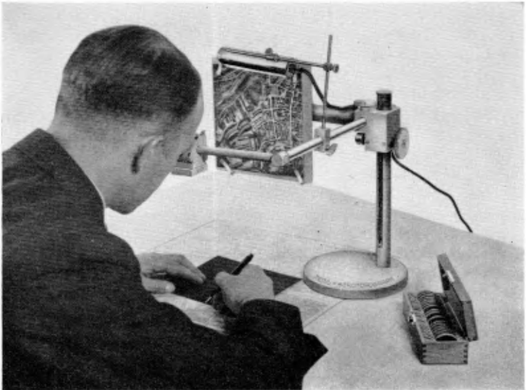
FIG. 7.4. ZEISS AERO-SKETCHMASTER (Zeiss Aerotopo)
