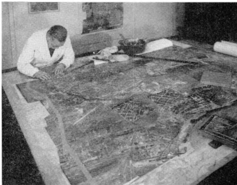
FIG. 7.20. A CONTROLLED MOSAIC UNDER CONSTRUCTION Note the registration with underlying map at left-hand edge. ( Hunting Surveys Ltd. )
