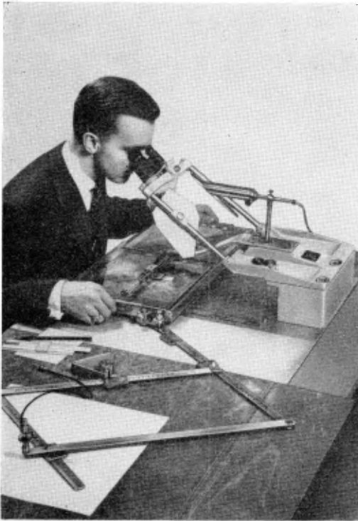
FIG. 7.15. THE STEREOPRET ( Zeiss Aerotopo )
