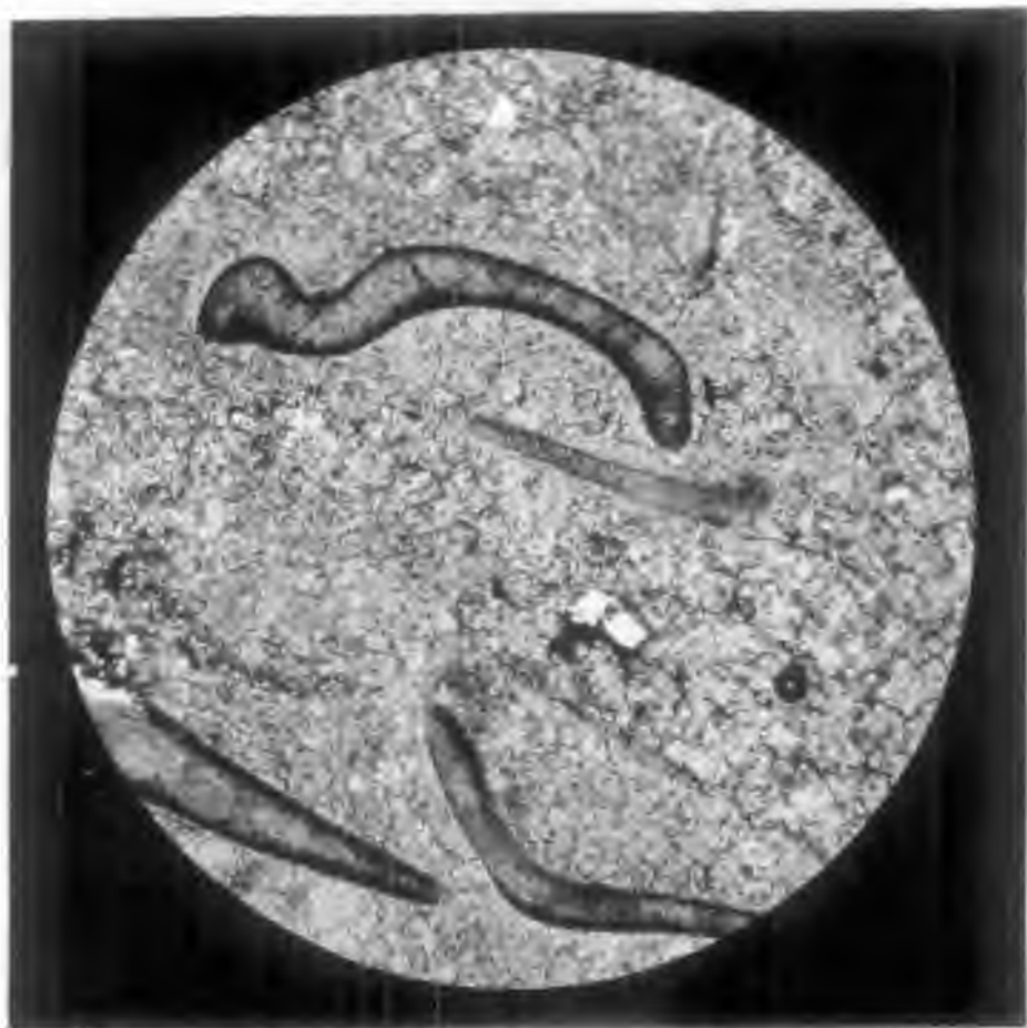
Fig. 17 Fossiliferous (shelly), microcrystalline dolomite (with trilobite frags). (X45); Hanson River Beds. Sample No. WB13, Neg. No. G/8738.
