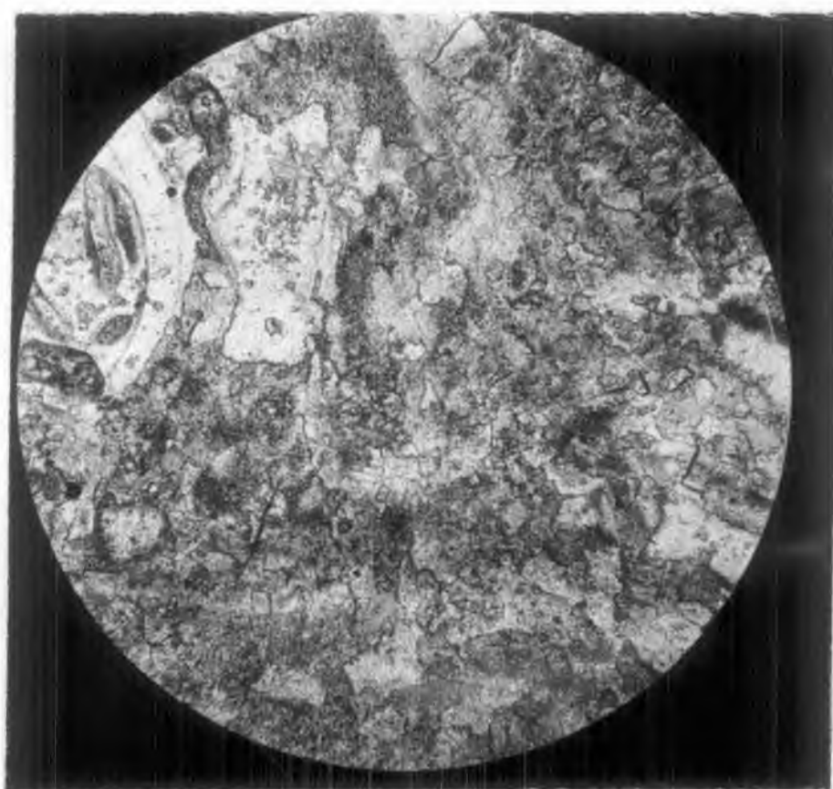
Fig. 11 Algal dolomite ( Girvanella? ) with bioclasts (X45), Merrina Beds. Sample No. WB1. Neg. No. G/8741
