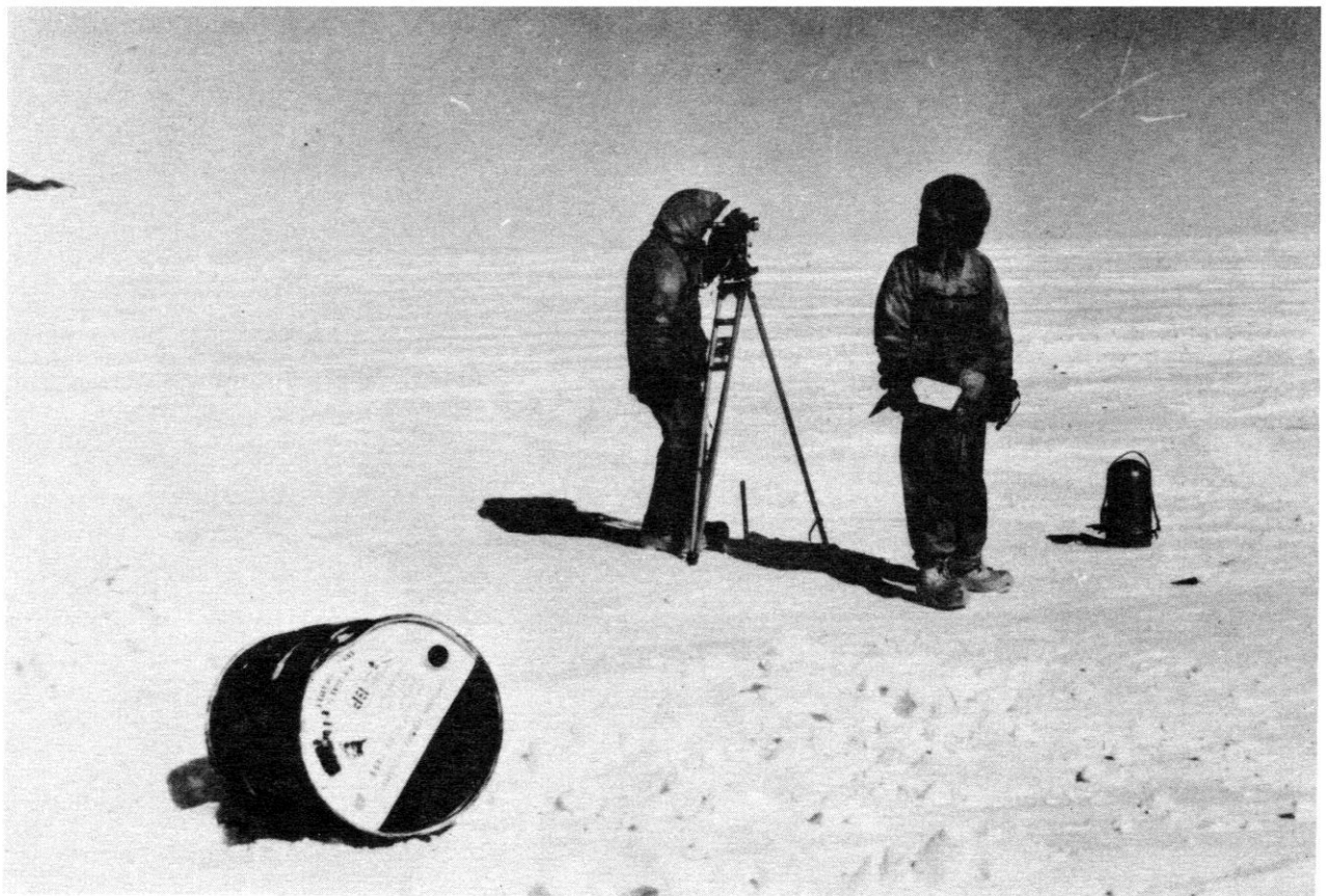
Angle observations on ice sheet, using Wild T3 theodolite
