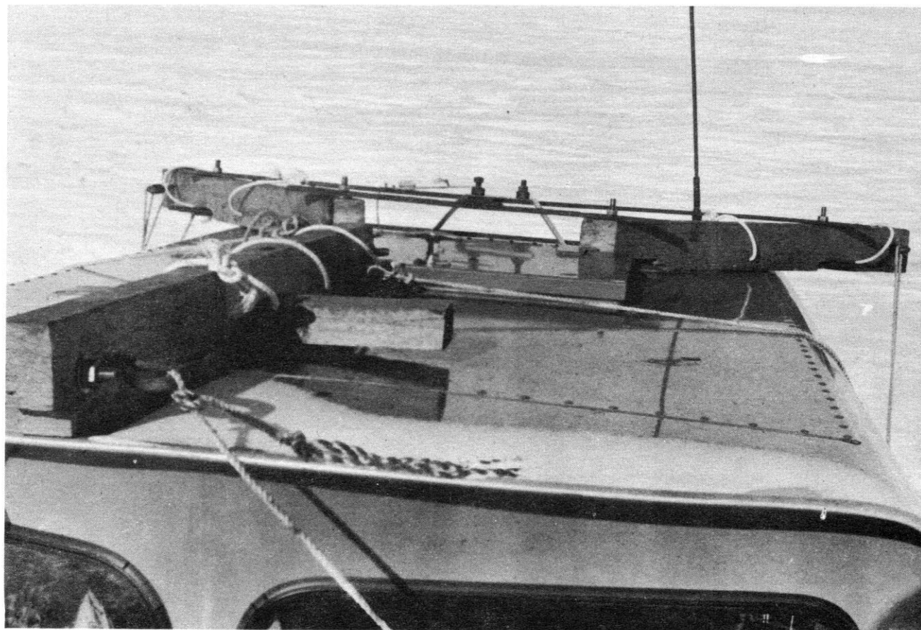
Adjustable rack for holding tripods on vehicle roof.
