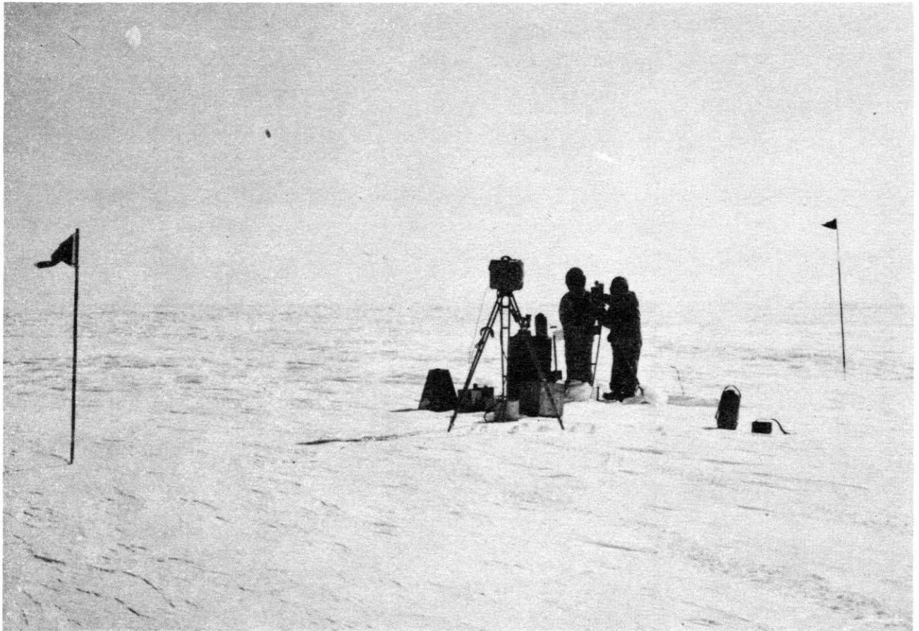
Typical ice station, showing station mark, drum, identifying canes and survey equipment.
